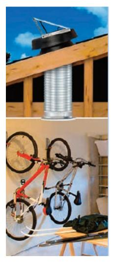
The Garage Exhaust Vent is an add-on kit that converts all Natural Light roof and curb mounted Solar Attic Fans into a garage ventilation system. An adapter sleeve is attached to the underside of the fan assembly and connected to a flexible duct pipe that runs through the attic. The kit includes an attractive white powder-coated ceiling vent that attaches to the garage ceiling. The systems venting capacity will depend on the model size of the solar attic fan and the length of flexible pipe used.
