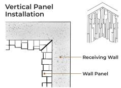
In the case of a vertical installation, a seamless internal corner is achieved by joining corresponding panels using a miter joint.
