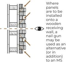
polymer adhesive. For best results, ensure that the appearance of the brads is minimized. When affixing wall panels above eye-level, brads should be "shot" at a downward angle. For panels below eye-level, shoot the brads at an upwards angle. Brads at eye-level should be shot into the corners of the panel and into the glue joints of the smaller wood blocks that comprise a panel.
