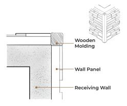
**Option 2:** Use a square piece of molding, running vertically, to join wall panels and create an outside corner with a special emphasis on the corner itself. We recommend that you use a complementary wood type and color for this solution.
