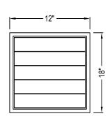
FRONT ELEVATION - INSULATED SIDING LOCKING POSITIONS 1/2", 3/4", 1", 1 1/4", 1 5/8"
