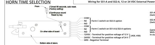
SS1-A Switch Rating: 1.0 A at 30 VDC (Switch is activated by the Push Bar)
