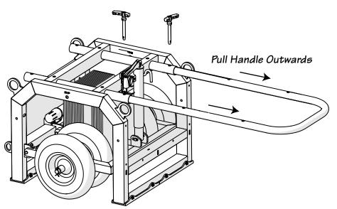
Pull the U shaped handle outward stopping when the last set of mounting holes is visual through the outer handle tube.
