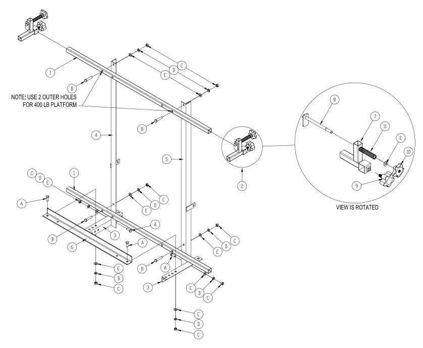
Figure 1B Assembly if Mounting onto 400 lb Carriage.
