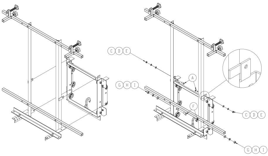
Figure 2 Mounting Solar Panel Carrier onto to Platform Carriage
