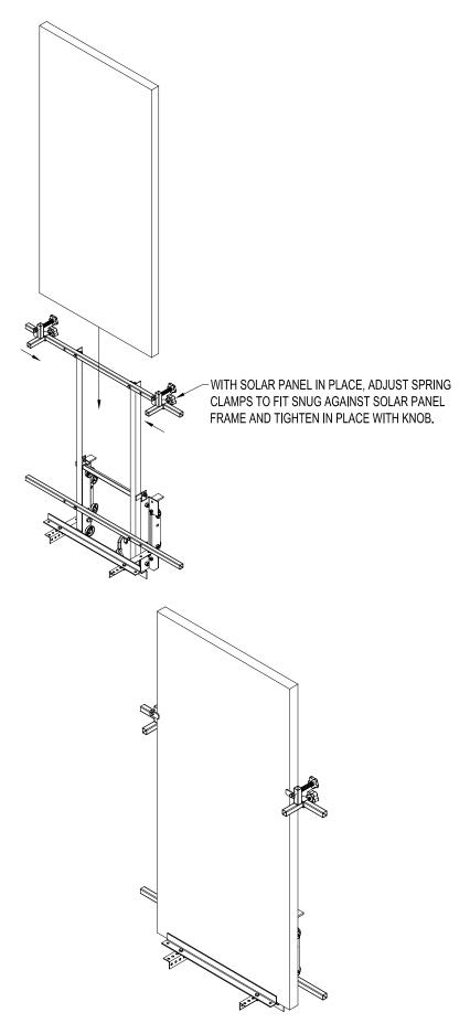
Figure 3 Placing Solar Panel onto Carrier
