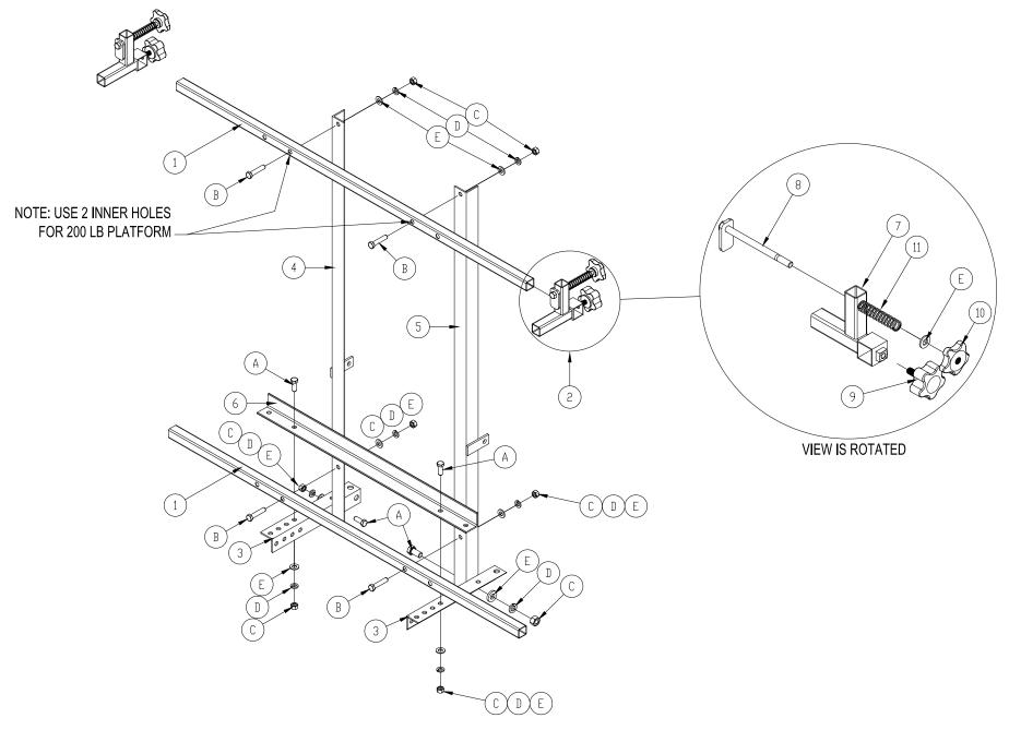
Figure 1A Assembly if Mounting onto 200 lb carriage.
