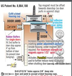
door and jamb to accept s/steel housing cups. (Recommended - Precision FB-23 Forstner Drill Bit)
