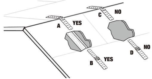
When multiple roof anchors are installed, the strength (static load) above must be met at each roof anchor's installation point independently.
