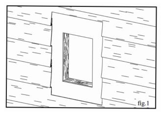
make the ring flexible so that it will slide between the siding and sheathing. Only cut through the nailing flange on the ring. Do not cut through the upright wall on the ring. See figure 2.
