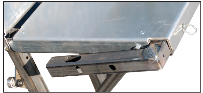
Plywood brackets in position for transport or storage.
