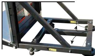
Insert Safety Pins from the inside of the carriage
