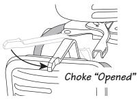
**Step 6 Running:** With the motor running, open (move to the right) the Choke lever.
