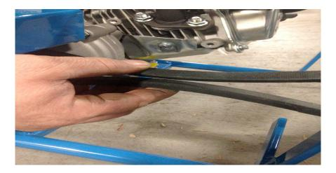
21. Attach the V-Belt by pushing it <u>over</u> belt guide bar, <u>between</u> the belt guard opening and then <u>looping</u> it over the engine drive pulley. See Figure 9. Figure9
