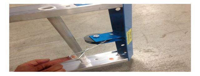
14. Attach the thimble on the cable to the back of carriage using the 1/2" bolt, nut and washers. Put 2 1/2" washers between thimble and carriage and 1 1/2" washer on other side of thimble. Pass the bolt thru the washers, thimble and then thru the bumper side angle then center hole on carriage. Tighten the 1/2" bolt so it passes thru the nut, but not so tight as to stop the thimble from rotating on the bolt. See Figure 7
