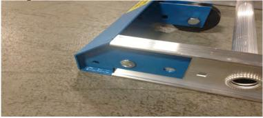
10. Slide the brake release handle over the brake bar and secure it with the hitch pin. See Figure 5
