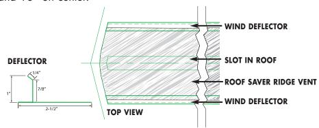
5. Install ridge cap shingles directly over Roof Saver®. Use galvanized roofing nails included in package to secure in place. When properly installed, Roof Saver® fills the 3/4" space between the underside of the cap shingle and the top surface of the roof shingles. Do NOT drive nails through shingle. **NAILS INCLUDED**
