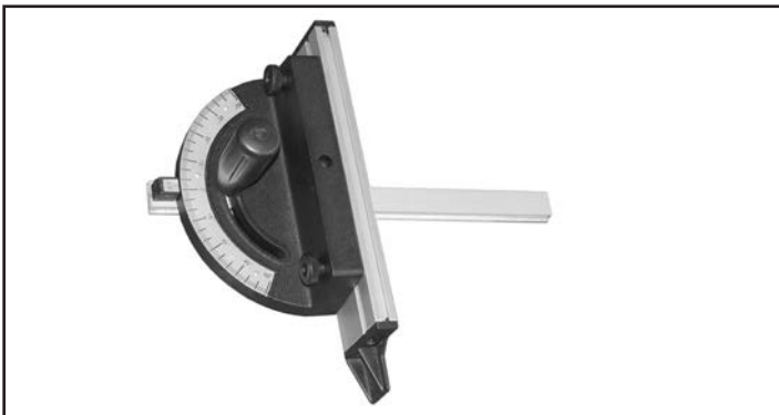
13-912 'T' SLOT MITER GAUGE Fits 3/4" x 3/8" miter slots. Handy scale for up to 60° left and right angle settings, includes adjustable 9" aluminium fence extension and push handle.
