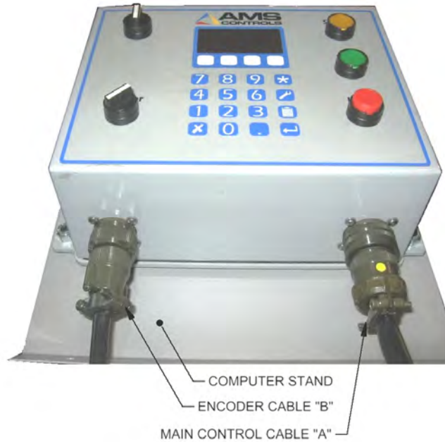
Figure 20: AMS Box With Cables
