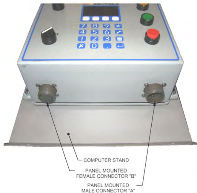
Figure 19: AMS Box Without Cables
