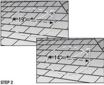
Hammer a nail at the center of the location chosen between rafters for the SolarAtticFan. The center of the unit should be about 2 feet down from the ridge.
