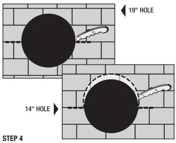
**19" HOLE:** With a razor knife, cut a four inch slit through the shingles and tar paper at the three and nine o'clock position of the flashing. This allows for the foot print of the flashing to be inserted under the shingles.
